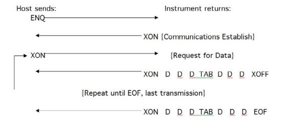
NOTE: When the data is being transferred to a host, the display on the instrument will flicker. This is an indication that serial communication is taking place.
