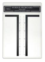
top to bottom. In the fourth subtest, the subject uses both hands alternately to construct "assemblies," which consist of a pin, a washer, a collar, and another washer. The subject must complete as many assemblies as possible within 1 minute.
