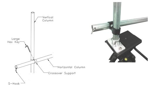
9. Attach the chain at the hook and below the tripod at the loop of cloth. The chain should cross under the tripod for maximum stability. The crossover fitting can be raised to make the chain more taught. To adjust the tripod, see the photos below. If it is difficult to keep steady, come back to this step once the Bassin Runway is attached.
